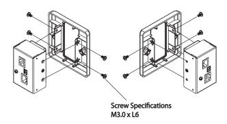
2. Screw the Wall Plate to the installation site (wall, ceiling, and so on).
