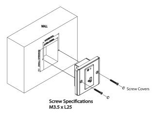
3. After making the necessary unit-to-unit Cat 5e cable connections, as well as the terminal block connection (optional), attach the Wall Plate Cover to secure and cover the VE157 / VE607 / VE807.
