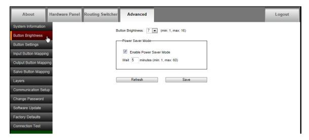
Button Brightness- The button brightness can be set to 16 different levels.
