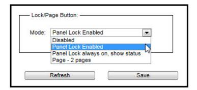
The "Lock" button on the front panel can also be used to change "pages" of operation.
