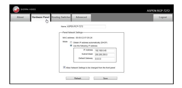
The front panel has the ability to change the network address. If you wish to disable this function, remove the check from the box "Allow Network Settings to be changed from the front panel".
