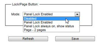
In this mode, this button will sequence through 2 pages of inputs and outputs. The button will have a different color for each page. The color for each page is also settable via the web page.
