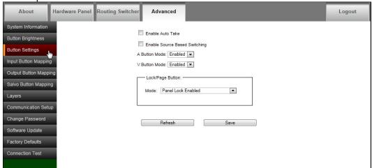
The control panel can be set for "Auto Take" mode. In the "Auto Take" mode, the routing switcher switches as soon a destination and source are selected (or a source and destination are selected if "Enable Source Based Switching" is selected (see below).
