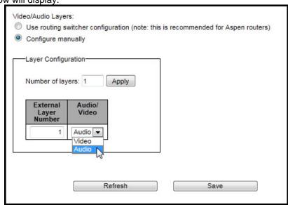
Enter the number of layers and hit Apply. Then select the signal type from the dropdown window and Save the configuration
