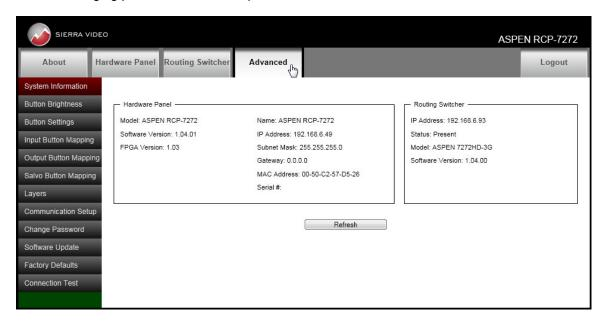
Clicking on the bars on the lefthand side of the screen gives access to adjustments and status.
