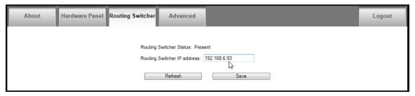
Make any changes necessary and press "Save" to implement changes. The control panel will need to be reset for these changes to take effect.
