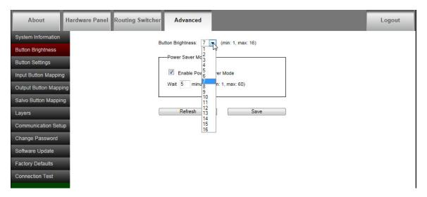
Power Saver Mode- When the Power Saver mode is enabled, the buttons will dim to 25% of the set brightness at the specified "wait" time.
