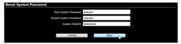
The password can also be changed from the "Advanced" tab (without entering the serial number).
