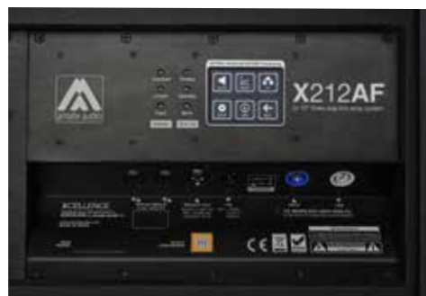
Connection Panel (Rear)
