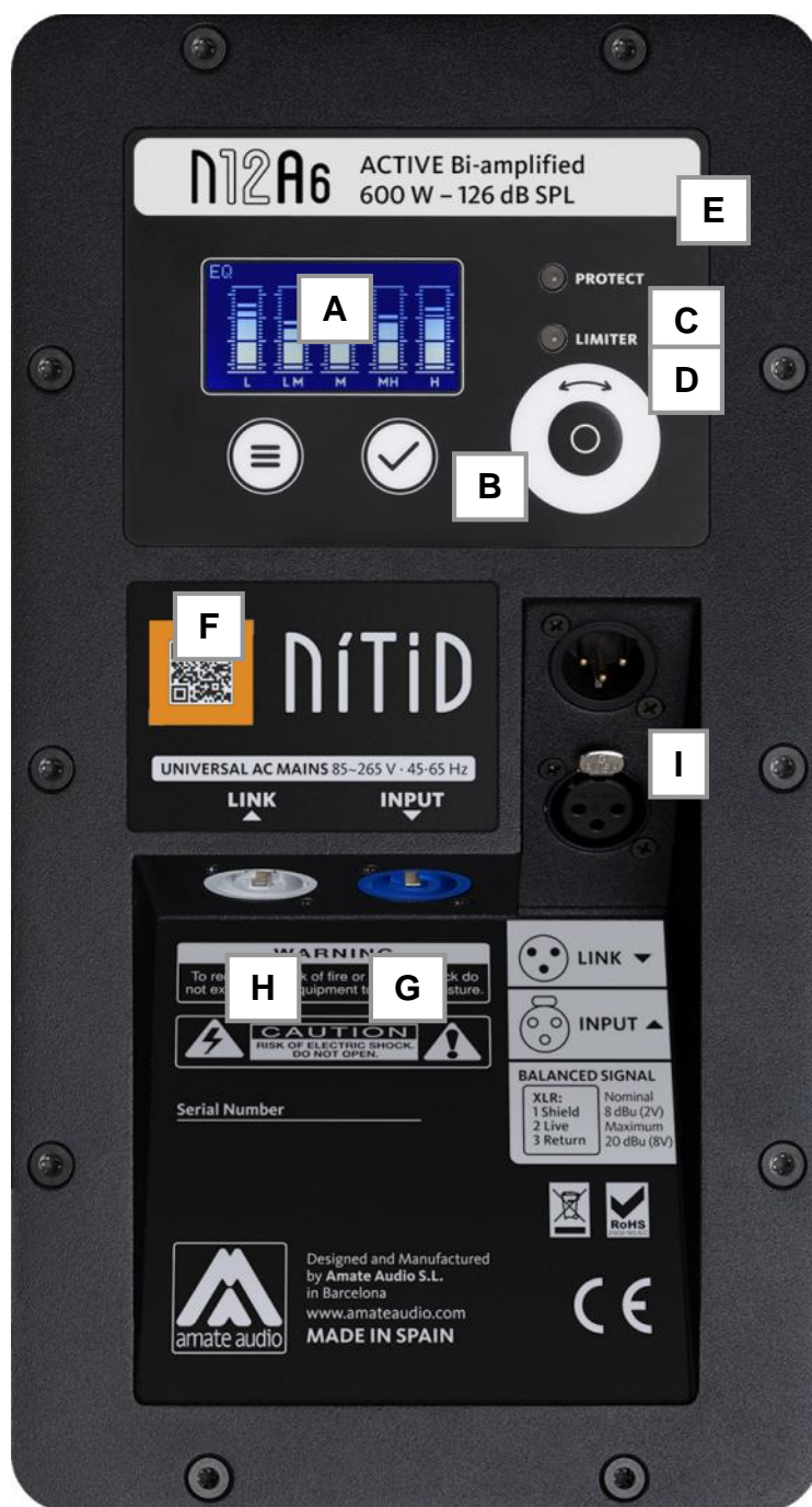
Fig. 2. N12A6 control and connection panel
