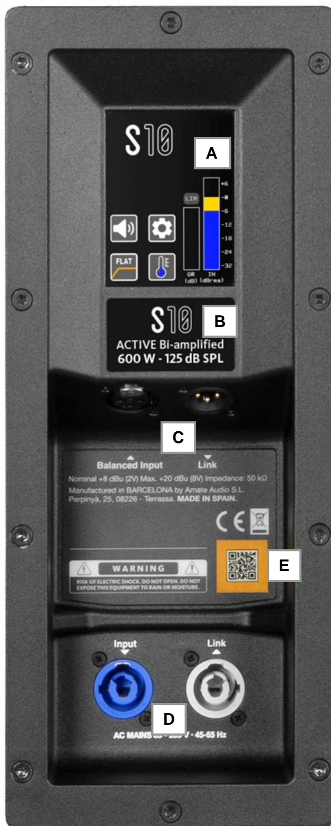
Fig. 2. S10 control and connection panel
