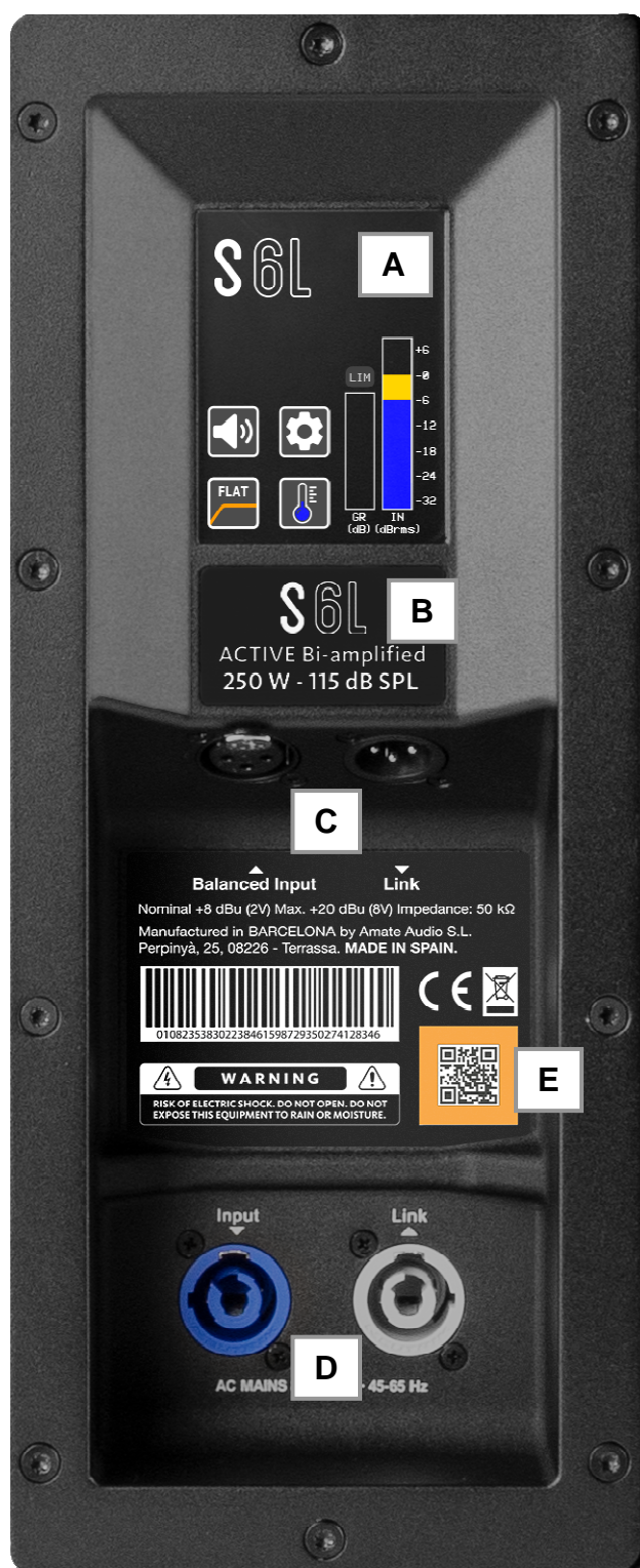
Fig. 2. S6L control and connection panel
