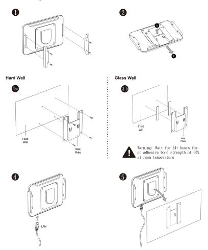
1. Secure the 2 LED bars onto the sides of the VK430 using the 4 LED bar screws provided.
