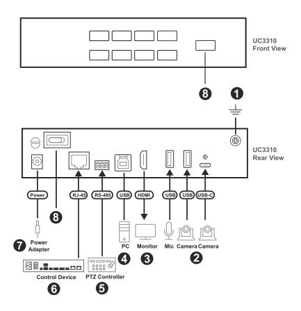
Ground the unit by connecting one end of a grounding wire to the grounding terminal and the other end to a suitable grounded object.
