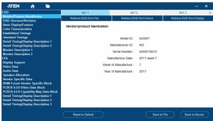
When you highlight the menu items, the right side panel displays the current settings for the corresponding EDID configuration. Some of the screens are read-only, including the following:
