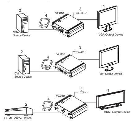
This completes the basic installation of the VGA/DVI/HDMI EDID Emulator. You may now power on the display and source devices.
