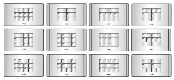
Custom button placement on the keypad can be set in 125 different combinations of 6 to 12 buttons. The example above shows the 12 most commonly used.
