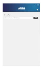
3. Wait for a few seconds for the app the scan for an available VP2020 / VP2021 device in the network environment.
