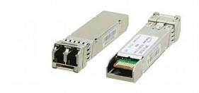
OSP-SM10 is a fiber optic transceiver for 1310nm single-mode signals. This standard pluggable SFP+ module has two LC connectors for reception and transmission signals over two strands of single-mode optical fiber
