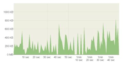
Slides with text and a few graphics are displayed on the **VIA** main display by a single connected client. Slides were advanced in irregular times to simulate real workflow.
