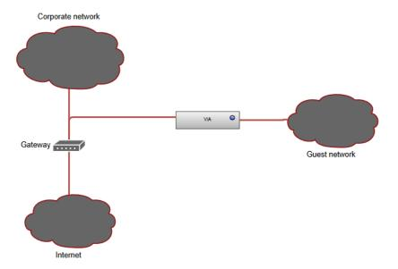
In this scenario, VIA is connected to both a corporate network (LAN 1) and a guest network (LAN 2). The corporate network is configured to assign a DHCP address with all related information. The guest network is not used by VIA to gain internet access or resolve domain names but is also configured to assign a DHCP address.
