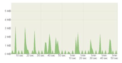
Slides consisting of heavy graphics and small animations are displayed on the **VIA** main display by a single connected client. Slides were advanced in irregular times to simulate real workflow.
