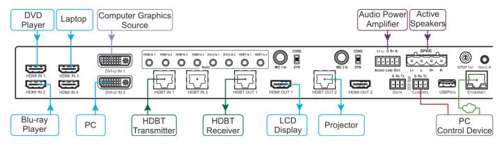
Note that you can connect DVI-U to an analog (VGA, composite or component video) or digital (HDMI or DVI) source.
